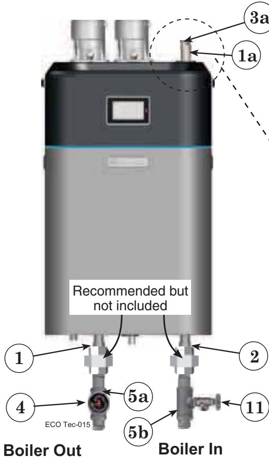
Figure 8 Install pipe fittings for relief valve and pressure/temperature gauge — DO NOT mount relief valve until AFTER hydrostatic testing (see legend below)
