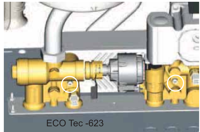
Figure 119 Removal of brazed plate heat exchanger by loosening the two (2) screws.
