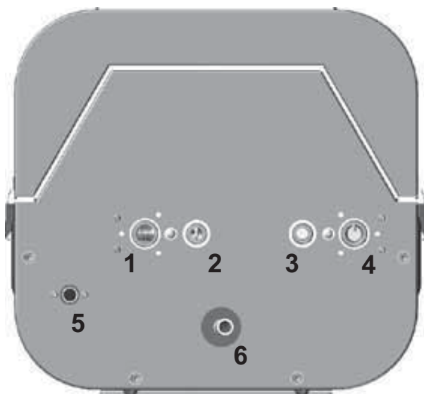
Figure 116 Boiler connections for cleaning domestic water circuit
